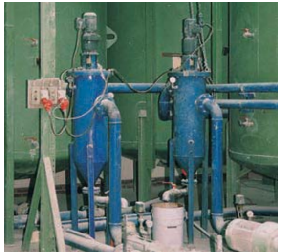
Automatic Metal Edge filter with scraper cleaning for adhesive
