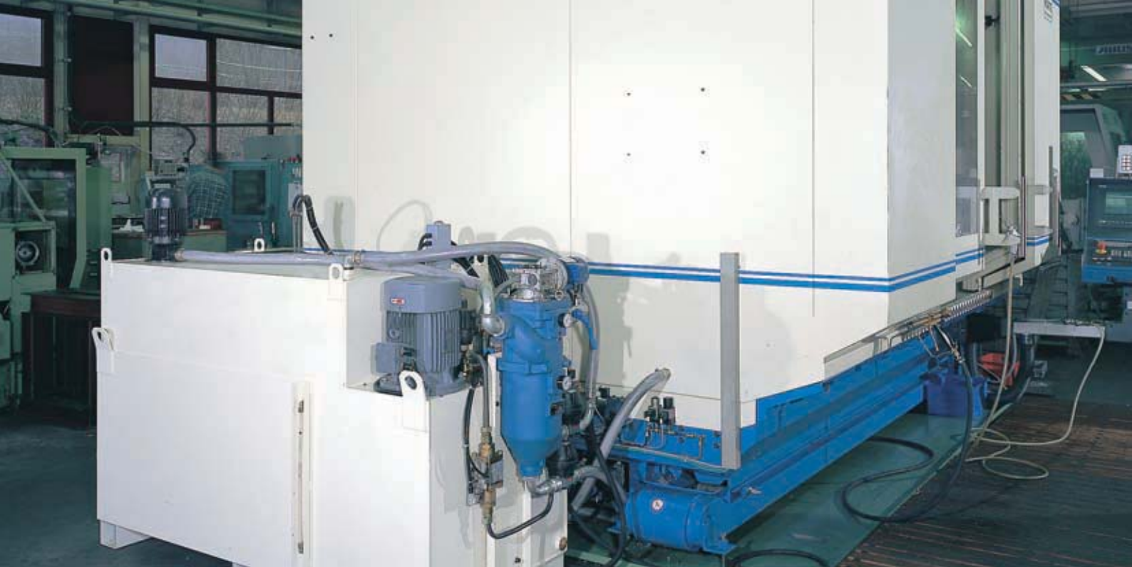
Automatic filter for cooling lubricant at a machining center
